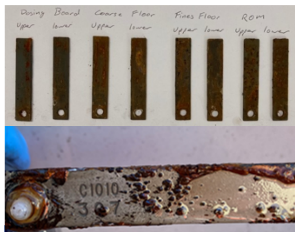
Corrosion coupons: (TOP) untreated, (BOTTOM) treated
