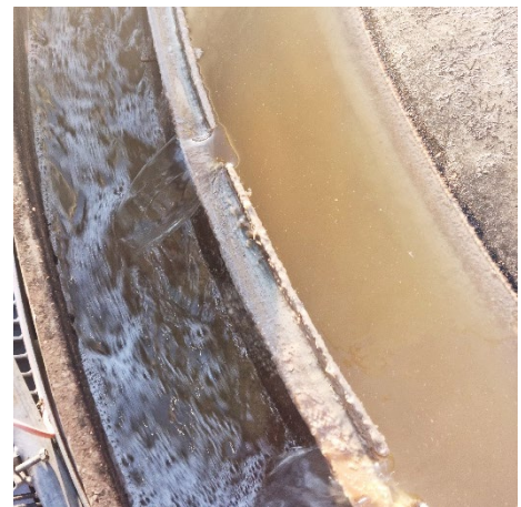
Clearer DAF effluent after application of WTS chemistry solutions
